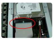
Connect to the E-IDE HDD cable
